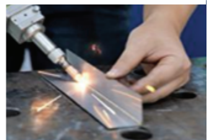
Corner iron diagonal welding
